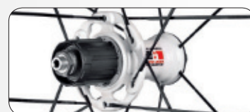
Oversized flange on the drive side
