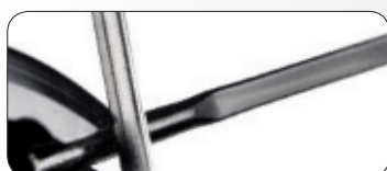
Double-butt steel spokes
