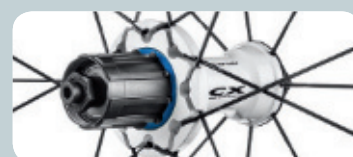
Oversized flange on the drive side
