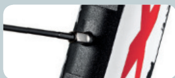
Nipples with self-locking system
