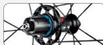
Oversized flange on the drive side
