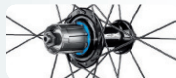
Oversized flange on the drive side
