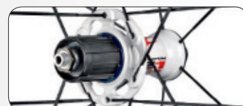
Oversized flange on the drive side
