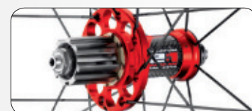
Oversized flange on the drive side
