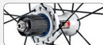
Oversized flange on the drive side
