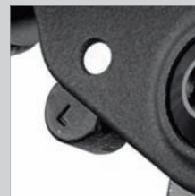
QUICK-RELEASE SYSTEM: it makes it easier to install and remove the wheel and allows, even during the race, to open the distance between the rim and the brake pads.
